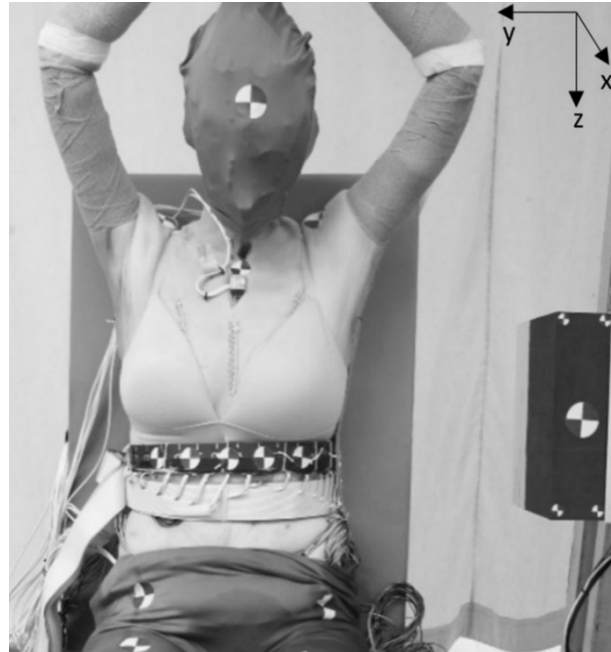
d) Initial PMHS seating posture and test set-up
