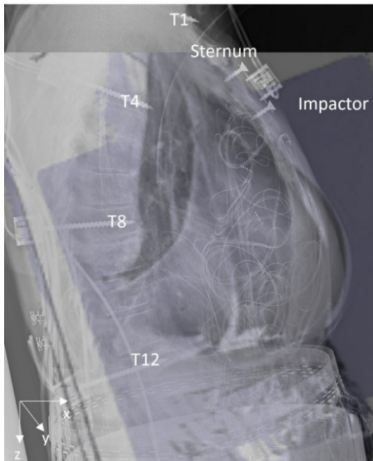
c) Faro scan and x-ray overlay showing impactor position
