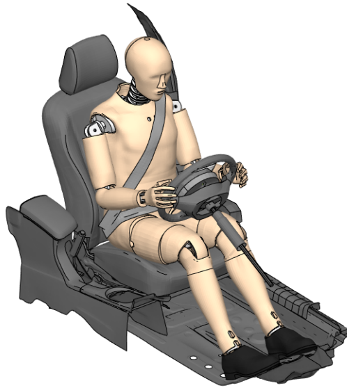
Figure 3: Initial positioning of the FE dummy in the driver seat configuration.
