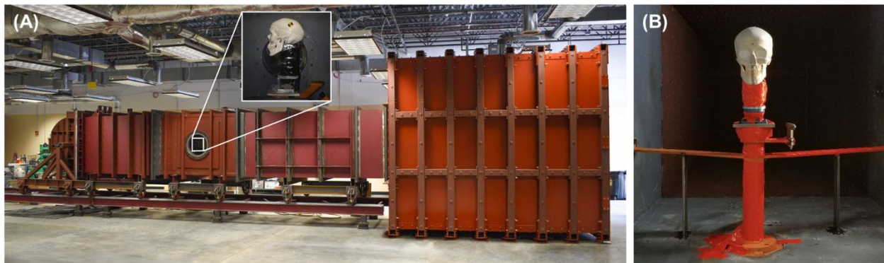
Figure 1: (A) A lateral view of the ABS4 at Virginia Tech with the mounting location of the headform highlighted and (B) the headform mounted to a stand in the center of the ABS4 test section.
