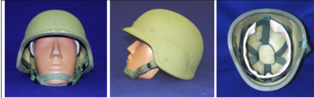
Figure 1: Prototype UHMWPE helmet used. Webbing suspension differs from newer pads often used in modern combat helmets. Adjustment is done by tensioning straps instead of pad removal.
