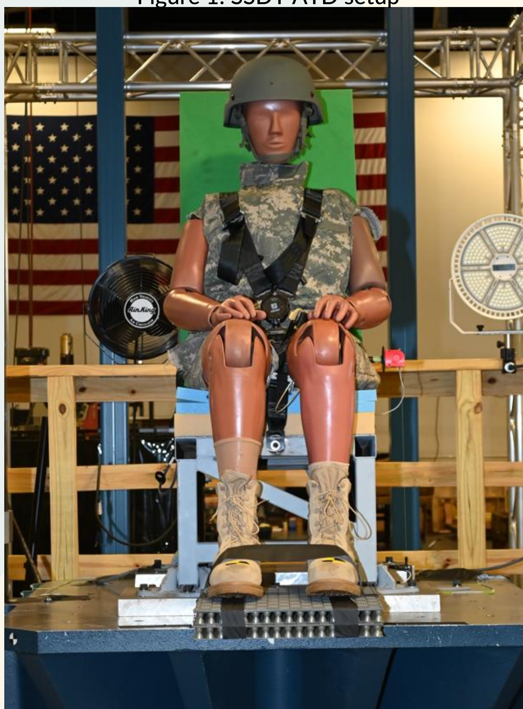
Figure 1: SSDT ATD setup
